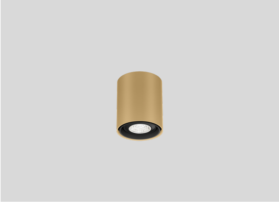
Cylindrical ceiling surface mounted downlight made from die-cast aluminium; surface Champagne; lamp socket GU10; lamp type PAR16; max. 12W; 100 - 240 V; degree of protection IP20; Class 1; UGR ≤ 19; inclusive single inner reflector in Black; lamp not included;
