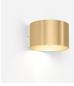
Cylindrical wall surface mounted luminaire made from aluminium; surface Champagne; direct light distribution; PCB 3-step binning; phase-cut dim; light colour 1800 K - 2850 K colour warm dimming; CRI  $\geq$  90; 220 - 240 V; degree of protection IP20; Class 1; inclusive flaps for adjustable beam angle; light source replaceable by Wever & Ducré or by a professional with explicit authorization;
