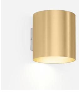
Cylindrical wall surface mounted luminaire made from aluminium; surface Champagne; direct/indirect light distribution; PCB 3-step binning; phase-cut dim; light colour 1800 K - 2850 K colour warm dimming; CRI  $\geq$  90; 220 - 240 V; degree of protection IP20; Class 1; driver included; inclusive flaps for adjustable beam angle; light source replaceable by an authorized professional;
