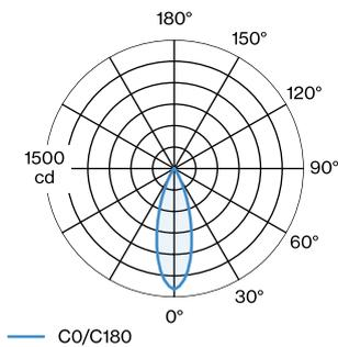
[186764W4', '911041G1'] The technical data represent rated values for an ambient temperature of 25°C. The data values for the luminous flux are initially subject to a tolerance of +/- 10%, those for the electrical connected load are initially subject to a tolerance of +/- 10%, and those for the colour temperature are initially subject to a tolerance of +/- 150 K. No liability is assumed for typographical or printing errors. The general terms and conditions of Wever & Ducré BV apply.
