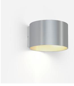
Cylindrical wall surface mounted luminaire made from aluminium; surface Aluminium Brushed; direct light distribution; PCB 3-step binning; phase-cut dim; light colour 2700 K; binning initial MacAdam  $\leq$ 3 SDCM; CRI  $\geq$  90; 220 - 240 V; degree of protection IP20; Class 1; inclusive flaps for adjustable beam angle; light source replaceable by Wever & Ducré or by a professional with explicit authorization;
