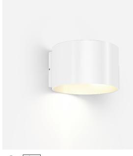
Cylindrical wall surface mounted luminaire made from aluminium; surface White Matt; powder coated; matt texture; RAL 9010; direct light distribution; PCB 3-step binning; phase-cut dim; light colour 2700 K; binning initial MacAdam  $\leq$  3 SDCM; CRI  $\geq$  90; 220 - 240 V; degree of protection IP20; Class 1; inclusive flaps for adjustable beam angle; light source replaceable by Wever & Ducré or by a professional with explicit authorization;
