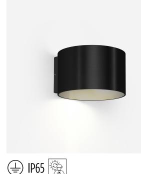
Cylindrical wall surface mounted luminaire made from aluminium; surface Black Matt; powder coated; matt texture; RAL 9005; direct light distribution; PCB 3-step binning; phase-cut dim; light colour 2700 K; binning initial MacAdam  $\leq$  3 SDCM; CRI  $\geq$  90; 220 - 240 V; degree of protection IP65; Class 1; inclusive flaps for adjustable beam angle; light source replaceable by Wever & Ducré or by a professional with
