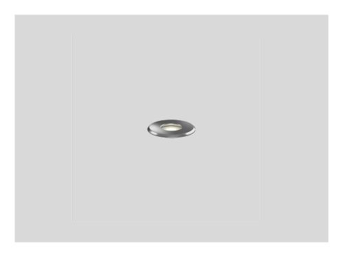
Round floor recessed luminaire made from stainless steel and glass; surface Inox; recessed depth 100 mm; with COB (Chip on Board) technology for maximum efficiency; phase-cut dim; light colour 3000 K; binning initial MacAdam  $\[ ]$ 3 SDCM; CRI  $\[ ]$ 90; beam angle 43°; degree of protection IP67; PC2; driver not included; light source replaceable by an authorized professional;
