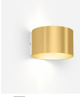
Cylindrical wall surface mounted luminaire made from aluminium; surface Gold; wet painted; brushed; direct/indirect light distribution; PCB 3-step binning; phase-cut dim; light colour 1800 K - 2850 K colour warm dimming; binning initial MacAdam  $\leq$  3 SDCM; CRI  $\geq$  90; 220 -240 V; degree of protection IP20; Class 1; driver included; inclusive flaps for adjustable beam angle; light source replaceable by Wever & Ducré or by a professional with explicit authorization;
