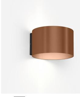
Cylindrical wall surface mounted luminaire made from aluminium; surface Copper; wet painted; brushed; direct/indirect light distribution; PCB 3-step binning; phase-cut dim; light colour 1800 K - 2850 K colour warm dimming; binning initial MacAdam  $\leq$  3 SDCM; CRI  $\geq$  90; 220 -240 V; degree of protection IP20; Class 1; driver included; inclusive flaps for adjustable beam angle; light source replaceable by Wever & Ducré or by a professional with explicit authorization;
