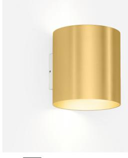
Cylindrical wall surface mounted luminaire made from aluminium; surface Gold; wet painted; brushed; direct/indirect light distribution; PCB 3-step binning; phase-cut dim; light colour 2700 K; binning initial MacAdam  $\leq$  3 SDCM; CRI  $\geq$  90; 220 - 240 V; degree of protection IP20; Class 1; driver included; inclusive flaps for adjustable beam angle; light source replaceable by an authorized professional;
