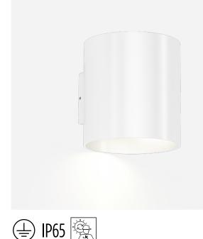
Cylindrical wall surface mounted luminaire made from aluminium; surface White Matt; powder coated; matt texture; RAL 9010; direct light distribution; PCB 3-step binning; phase-cut dim; light colour 2700 K; binning initial MacAdam  $\leq$  3 SDCM; CRI  $\geq$  90; 220 - 240 V; degree of protection IP65; Class 1; inclusive flaps for adjustable beam angle; light source replaceable by Wever & Ducré or by a professional with explicit authorization;
