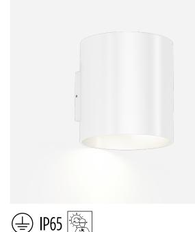
Cylindrical wall surface mounted luminaire made from aluminium; surface White Matt; powder coated; matt texture; RAL 9010; direct light distribution; PCB 3-step binning; phase-cut dim; light colour 3000 K; binning initial MacAdam  $\leq$  3 SDCM; CRI  $\geq$  90; 220 - 240 V; degree of protection IP65; Class 1; inclusive flaps for adjustable beam angle; light source replaceable by Wever & Ducré or by a professional with explicit authorization;
