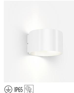
Cylindrical wall surface mounted luminaire made from aluminium; surface White Matt; powder coated; matt texture; RAL 9010; direct/ indirect light distribution; PCB 3-step binning; phase-cut dim; light colour 2700 K; binning initial MacAdam  $\leq$  3 SDCM; CRI  $\geq$  90; 220 -240 V; degree of protection IP65; Class 1; inclusive flaps for adjustable beam angle; light source replaceable by Wever & Ducré or by a professional with explicit authorization;
