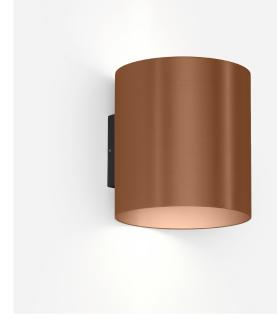
Cylindrical wall surface mounted luminaire made from aluminium; surface Copper; wet painted; brushed; direct/indirect light distribution; PCB 3-step binning; phase-cut dim; light colour 3000 K; binning initial MacAdam  $\leq$  3 SDCM; CRI  $\geq$  90; 220 - 240 V; degree of protection IP20; Class 1; driver included; inclusive flaps for adjustable beam angle;
