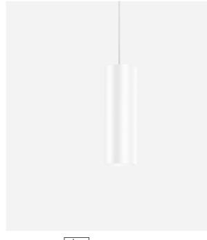
Cylindrical ceiling suspended luminaire made from die-cast aluminium; surface White Matt; powder coated; matt texture; inclusive adjustable cable suspension max. 4000mm in Pure White; with COB (Chip on Board) technology for maximum efficiency; light colour 1800 K - 3000 K colour warm dimming; CRI  $\geq$  90; 24 V; degree of protection IP20; Class 3; driver included; ceiling base included; light source replaceable by Wever & Ducré or by a professional with explicit authorization;
