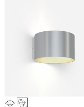
Cylindrical wall surface mounted luminaire made from aluminium; surface Aluminium Brushed; direct/indirect light distribution; PCB 3step binning; light colour 1800 K - 3000 K colour warm dimming; CRI  $\geq$  90; 24 V; degree of protection IP20; Class 3; driver included; inclusive flaps for adjustable beam angle; light source replaceable by Wever & Ducré or by a professional with explicit authorization;
