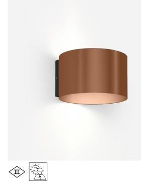
Cylindrical wall surface mounted luminaire made from aluminium; surface Copper; wet painted; brushed; direct/indirect light distribution; PCB 3-step binning; light colour 1800 K - 3000 K colour warm dimming; CRI  $\geq$  90; 24 V; degree of protection IP20; Class 3; driver included; inclusive flaps for adjustable beam angle; light source replaceable by Wever & Ducré or by a professional with explicit authorization;
