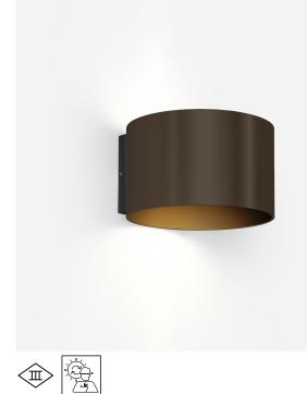
Cylindrical wall surface mounted luminaire made from aluminium; surface Bronze; wet painted; brushed; direct/indirect light distribution; PCB 3-step binning; light colour 1800 K - 3000 K colour warm dimming; CRI  $\geq$  90; 24 V; degree of protection IP20; Class 3; driver included; inclusive flaps for adjustable beam angle; light source replaceable by Wever & Ducré or by a professional with explicit authorization;
