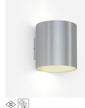
Cylindrical wall surface mounted luminaire made from aluminium; surface Aluminium Brushed; direct/indirect light distribution; PCB 3step binning; light colour 1800 K - 3000 K colour warm dimming; CRI  $\geq$  90; 24 V; degree of protection IP20; Class 3; driver included; inclusive flaps for adjustable beam angle; light source replaceable by an authorized professional;
