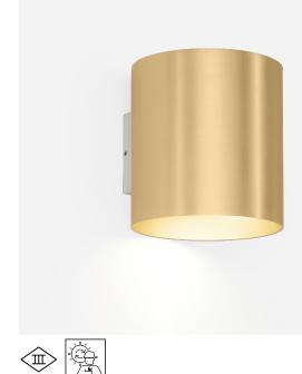
Cylindrical wall surface mounted luminaire made from aluminium; surface Champagne; direct/indirect light distribution; PCB 3-step binning; light colour 1800 K - 3000 K colour warm dimming; CRI  $\geq$  90; 24 V; degree of protection IP20; Class 3; driver included; inclusive flaps for adjustable beam angle; light source replaceable by an authorized professional;
